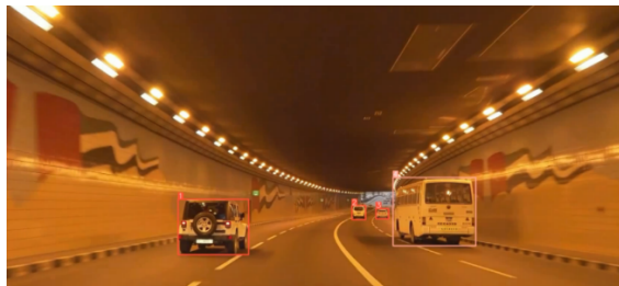
Figure 6: Effect of Vehicle Detection Based on YOLOv5-s int8 Quantization [from internet].
